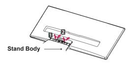
3 Remove the two screws on the back of stand body.
