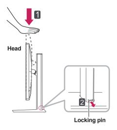
3 The height can be adjusted up to 110.0 mm.
