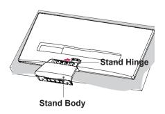
4 Tighten two screws into the back of the stand body.
