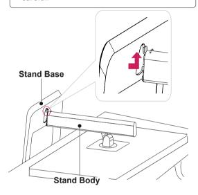
3 Fix by turning the screw to the right with a coin.
