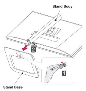
3 Remove the two screws from the stand body.
