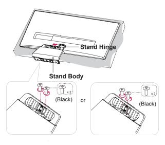
4 Remove the two screws from the Stand Base.
