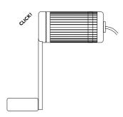
2 Slide crank handle into the groove and wait for a click.
