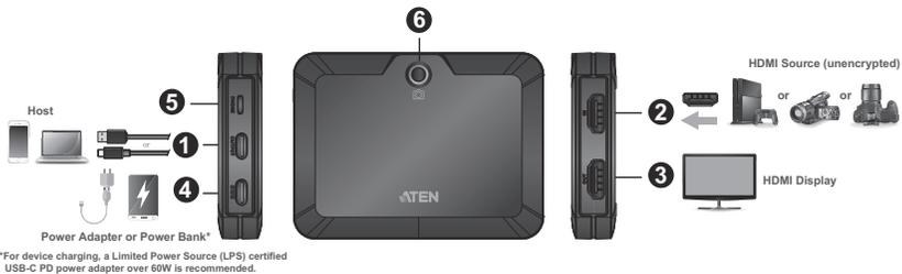
1. Connect the USB-C UVC output port to a host (e.g. laptop or Android Phone) using the USB-C to USB-C cable<sup>1</sup> (included). Or, if your laptop only has a USB-A interface, connect the USB-C to USB-A cable (included) to the host.
