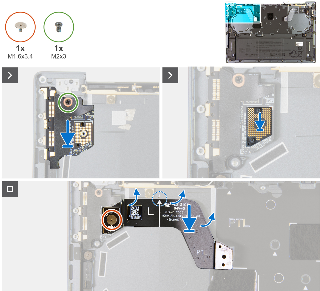
Figure 38. Installing the left I/O daughterboard
