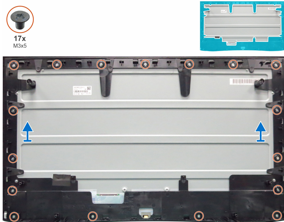
Figure 21. Removing the middle frame for S2725HSM
