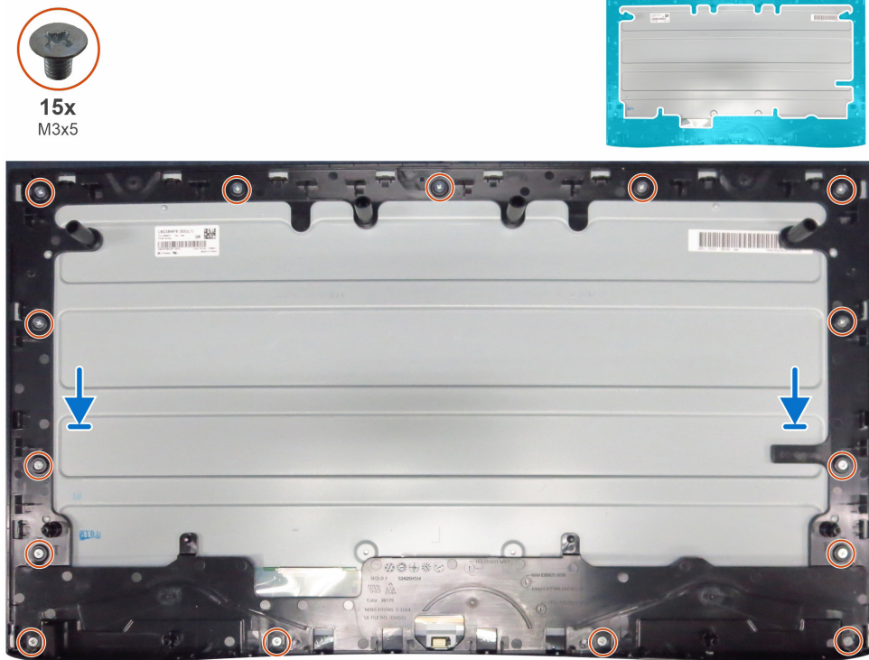
Figure 22. Installing the middle frame for S2425HSM
