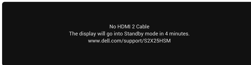
Figure 29. HDMI 2 cable disconnected warning message
