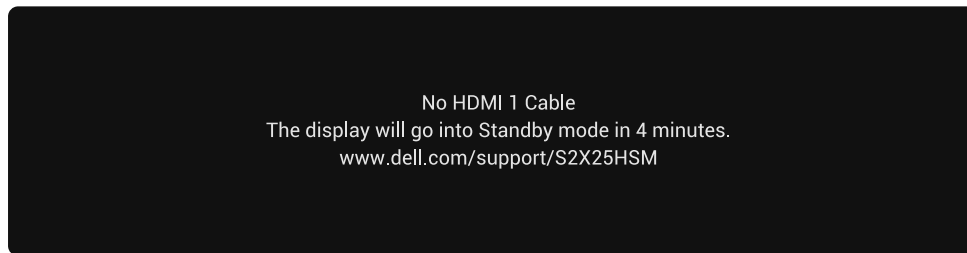
Figure 28. HDMI 1 cable disconnected warning message
