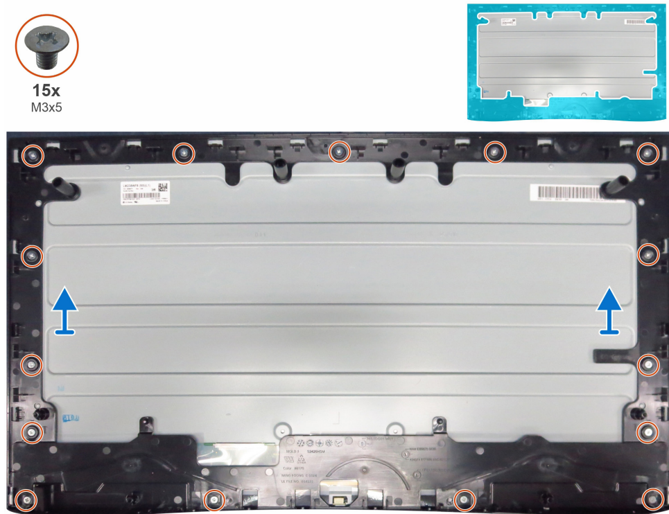
Figure 20. Removing the middle frame for S2425HSM
