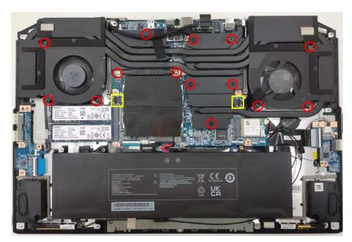
4.Unlock the RAM and take out the RAM. Unfasten fourteen screws of the FAN and the thermal module. Disconnect the cable of the Fan then remove them
