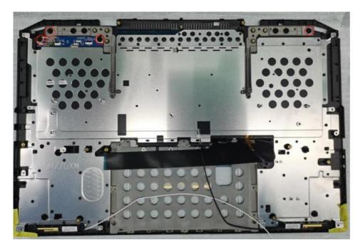
7. Unfasten four screws &cable. Then take out the Power board
