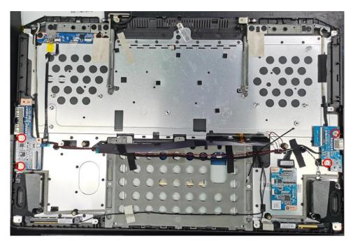
6. Unfasten four screws &cable. Then take out the USB board & audio board
