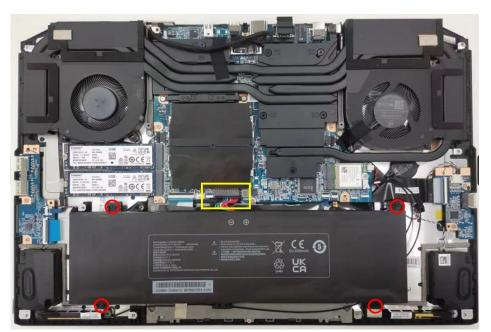
2. Unfasten Battery cable and Unfasten four battery screws then pull out the battery.
