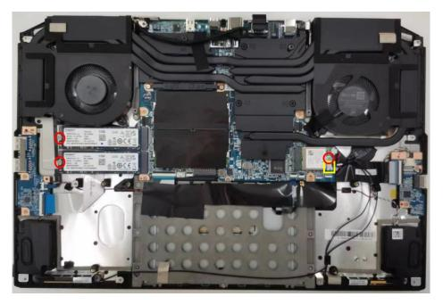
3. Unfasten three screws disconnect the wlan antenna. take out the SSD,WLAN
