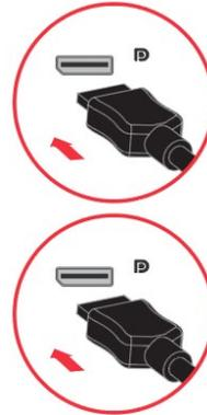
4. Connect one end of the HDMI 2.0 cable to the HDMI connector on the back of the computer, and the other end to the HDMI connector on the monitor. Lenovo recommends that customers who require to use the HDMI input on their monitor purchase the "Lenovo HDMI to HDMI cable OB47070".
