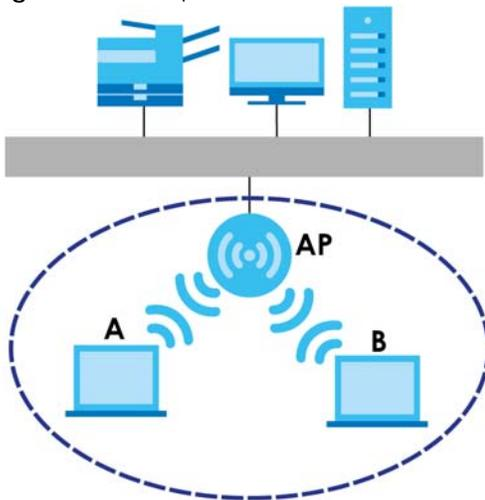
The wireless network is the part in the blue circle. In this wireless network, devices **A** and **B** are called wireless clients. The wireless clients use the access point (AP) to interact with other devices (such as the printer) or with the Internet. Your LTE2566-M634 is the AP.
