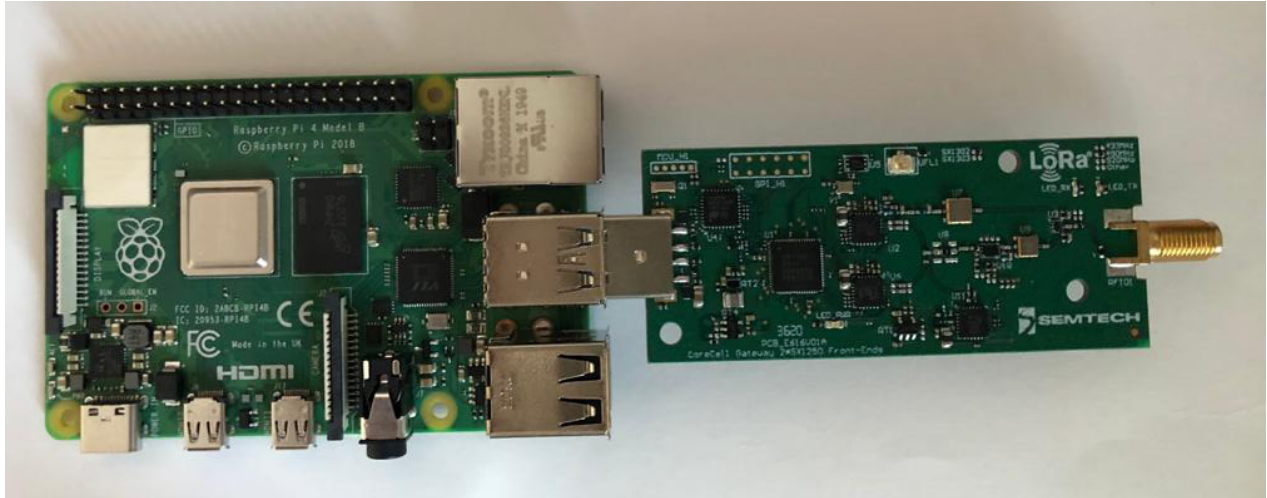
Figure 8: LoRa Corecell GW, Interface Board & Raspberry Pi Connection (CN490)
