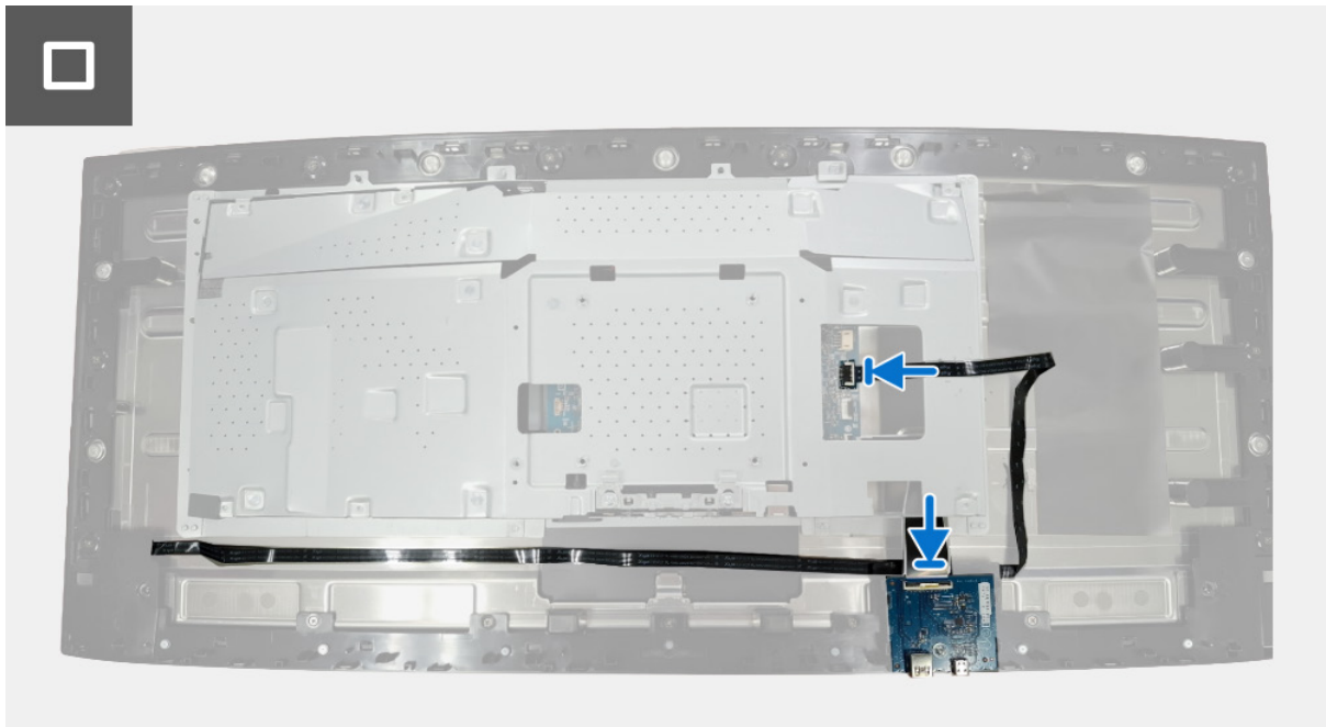
Figure 20. Installing the metal shield
