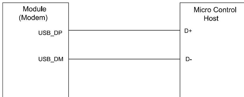
Figure 3-10 Recommended circuit of USB interface
