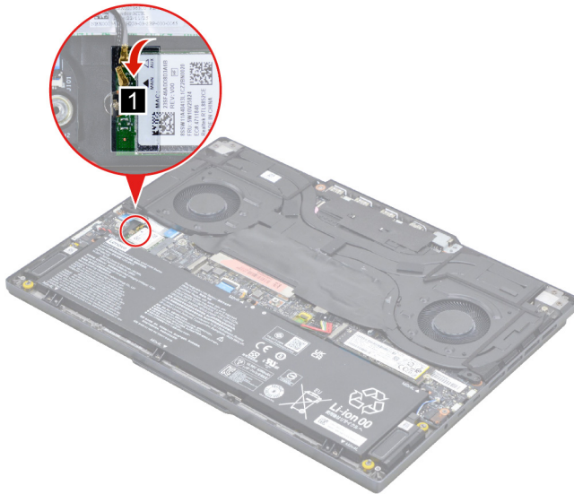
Figure 10. Peel off the Wi-Fi card mylar
