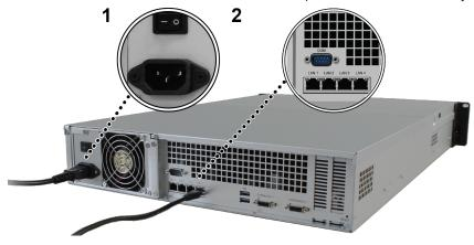
3 Make sure the Power Supply On/Off Switch is turned on ("|").
