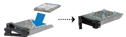
3 Insert the loaded drive tray into the empty hard drive bay.
