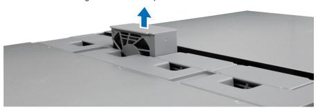
**5** Prepare a new fan, and slide it into the RackStation. Make sure the fan is aligned properly as illustrated below.
