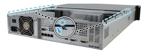
**b** Put back and fasten the screw you removed in step 2-a.
