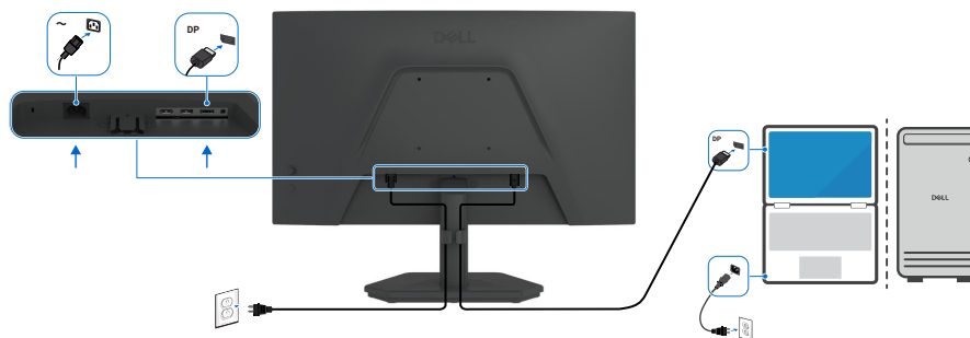
Figure 9. Connecting the DisplayPort cable
