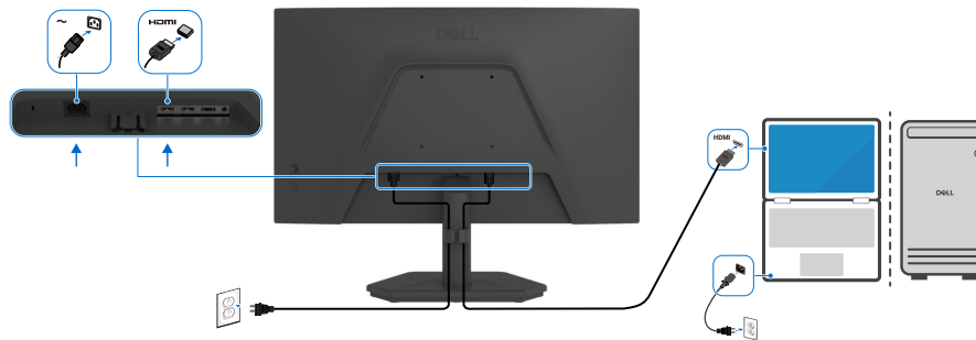
Figure 8. Connecting the HDMI Cable
