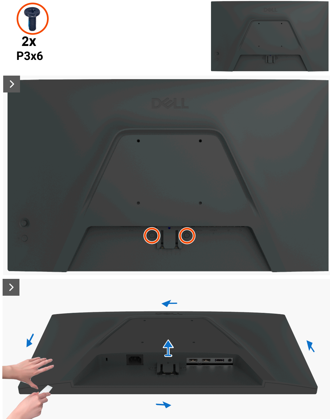
Figure 14. Removing the back cover
