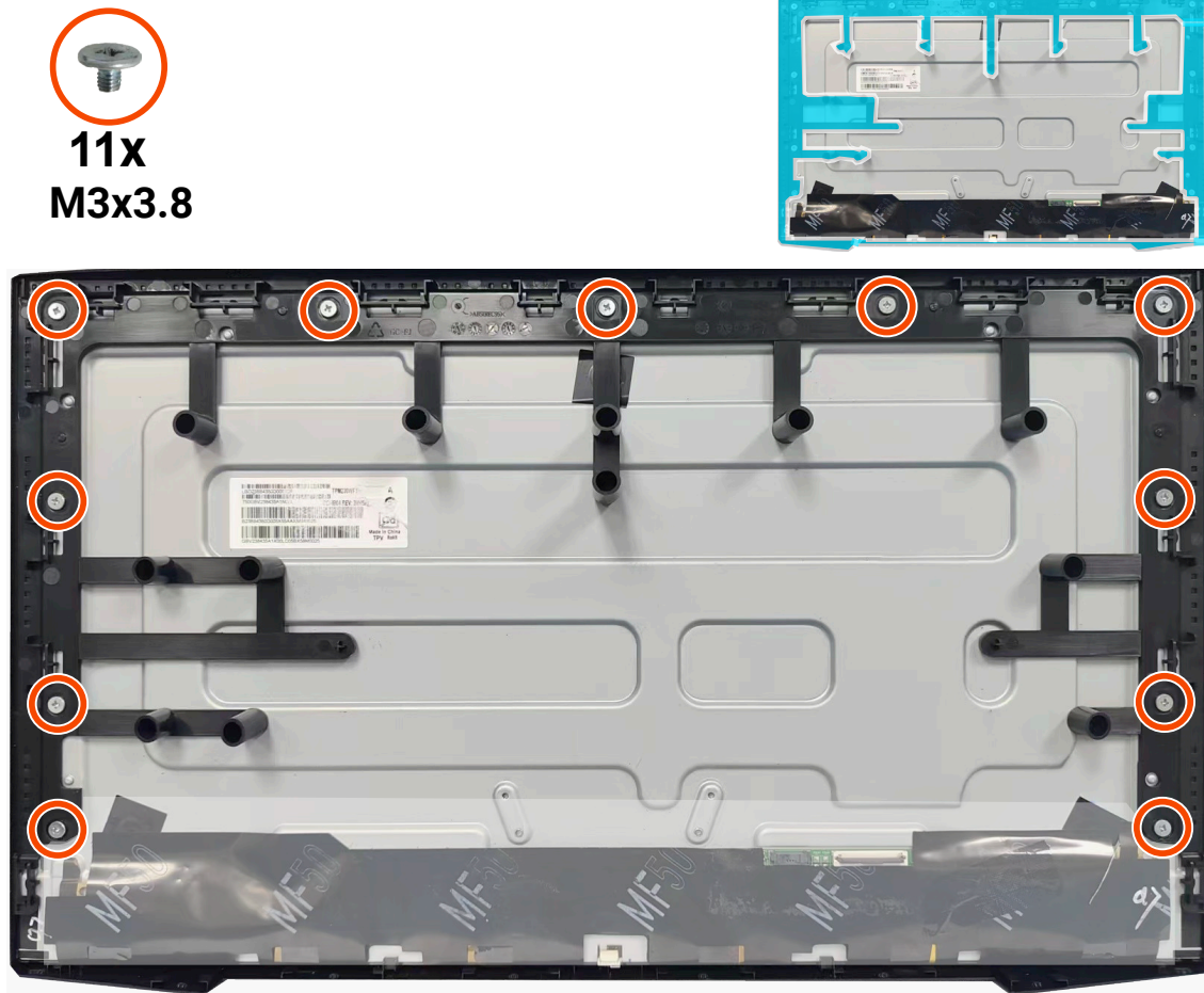
Figure 29. Installing the middle frame
