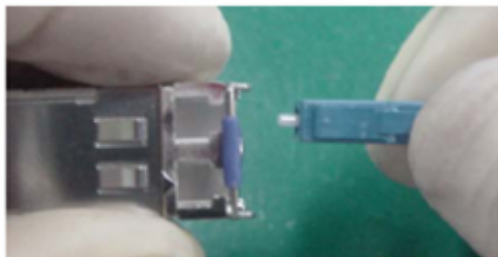
Figure 9-98 Using fibers to protect an optical module
