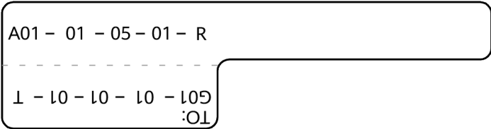
Figure 9-89 Sample label on an optical fiber between two devices
