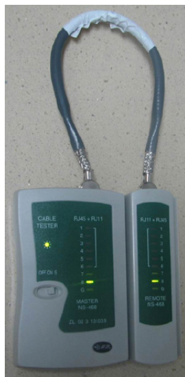
Figure 9-39 Testing the conduction and connections of wires
