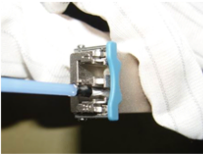
Figure 9-100 Cleaning a receptacle with a cotton swab
