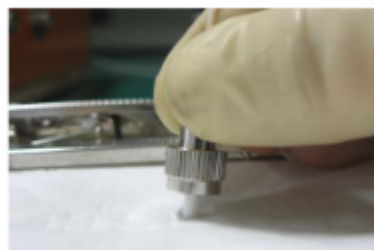
Figure 9-96 Cleaning optical fibers with special cleaning tissues
