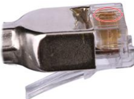
Figure 9-34 Unparallel contact strips of different heights
