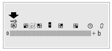
In the display  ${\bf c}$  and  ${\bf l}$  alternately light up and  ${\bf l}$  lights up as a default setting.
