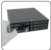
Slide the key lock to the left until the handle comes out and release the tray
