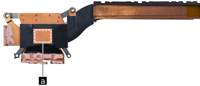
Figure 13. Areas on the heat sink where thermal interface materials should be applied
