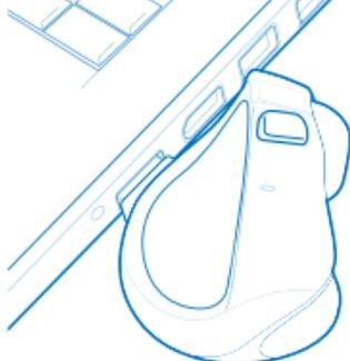
The battery LED will flash green while charging and turns off once fully charged. The first 60 seconds of charging will give up to one hour of use. A full charge can take up to 90 minutes, giving up to 2 weeks of use. To begin using the mouse, move the switch on the underside to the **ON** position
