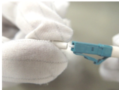
Figure 13-47 Installing a protective cap on a fiber
