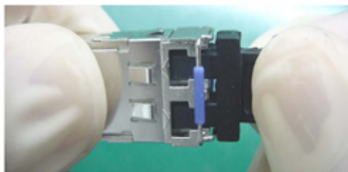
Figure 13-45 Installing a protective cap
