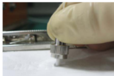
Figure 13-44 Cleaning optical fibers with special cleaning tissues
