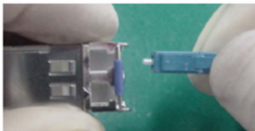
Figure 13-46 Using fibers to protect an optical module
