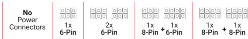
If your card has 2 power connections, BOTH need to be connected, graphics cards will not work if only 1 out of 2 power connections is plugged in. Any red lights near the power connectors indicate some sort of power related issue.
