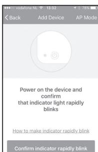
7. As soon as the light on the device flashes quickly, select in the app: «Confirm Indicator rapidly blinks». If the device has already been connected to the WiFi modem, the WiFi Light will not blink automatically.
