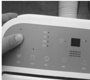
Press and hold the Power button for 5-10 seconds, then press the SLEEP button until you hear a tone and see the WiFi light blink rapidly.
