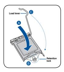
Insert the load lever under the retention tab to remove the PnP cap from the CPU socket.
