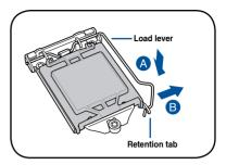
Lift the load lever until the load plate is completely lifted.
