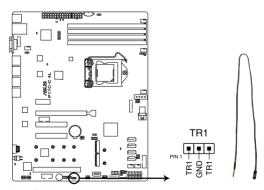
P11C-E 4L Thermal sensor cable connector
