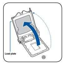
Position the CPU above the socket, ensuring that the gold triangle mark is on the bottom-left corner of the socket, then fit the CPU notches to the socket's alignment keys.
