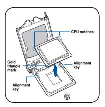
Close the load plate (A), ensuring that the front edge of the load plate slides under the retention lock (B) then push down the load lever (C).
