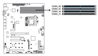
P11C-E/4L 288-pin DDR4 DIMM sockets
