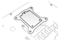
Use a Phillips screwdriver to tighten the four heatsink screws using the recommended sequence below.
