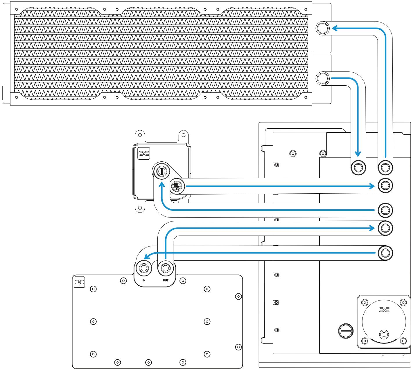
If more than 3 components are to be connected (e.g. another radiator), the setup can look as shown.
