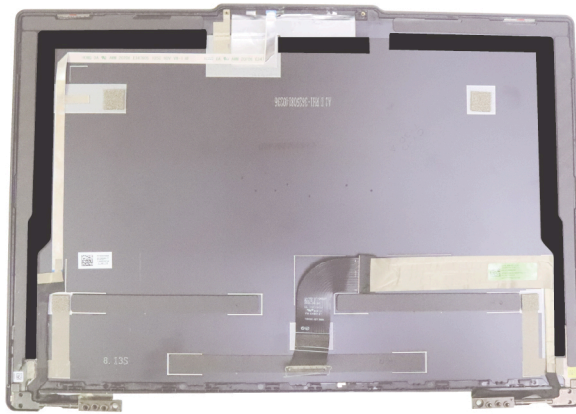
Figure 59. The locations where the stretch release tapes should be attached
