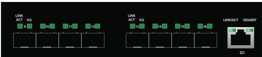
**TIP** The default stack ports on the 500X are XG3/S1 and XG4/S2. If the correct module is plugged into XG3/S1 and XG4/S2, the switch should be able to detect the connection and configure the speed according to the module capability without any manual configuration. The 5G/S1 and 5G/S2 interfaces on the 500X need to be configured manually via the CLI or web-based interface in order to utilize these ports as stack ports.
