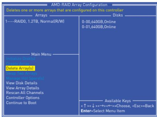
2. Select the arrays to delete by pressing **Insert** key.
