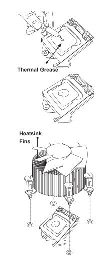
Recommended Supermicro heatsink: SNK-P0046A4 or SNK-P0051AP4 active heatsink (2U+ or 4U chassis)
