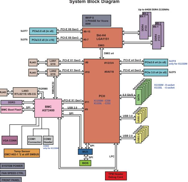
Figure 1-4. System Block Diagram
