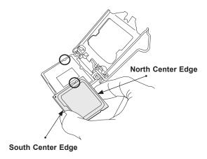
4. Align the CPU key that is the semi-circle cutouts against the socket keys. Once it is aligned, carefully lower the CPU straight down into the socket. (Do not drop the CPU on the socket. Do not move the CPU horizontally or vertically.
