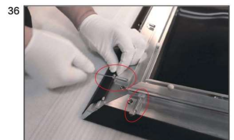
( 36-37 Make sure the springs is align the holes of the fabric. Two person Please install the two springs which is closing to the corners. at the same time ( show as pic) )
