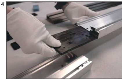
( 4 silver frame install: first step combine the two piece of short silver frame with the connection parts. )
