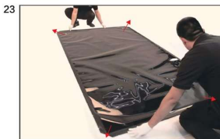
(23 pull the fabric on both sides at the same time, to make sure the fabric is basically flat)
