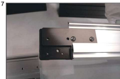
( 4 silver frame install: first step combine the two piece of short silver frame with the connection parts. )
