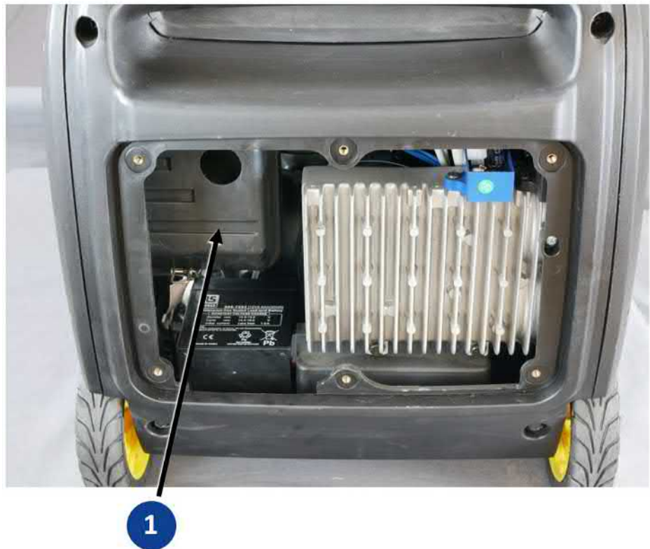
Fig. 9-5 Luftfilter bakom ventilationsgaller (borttaget)
