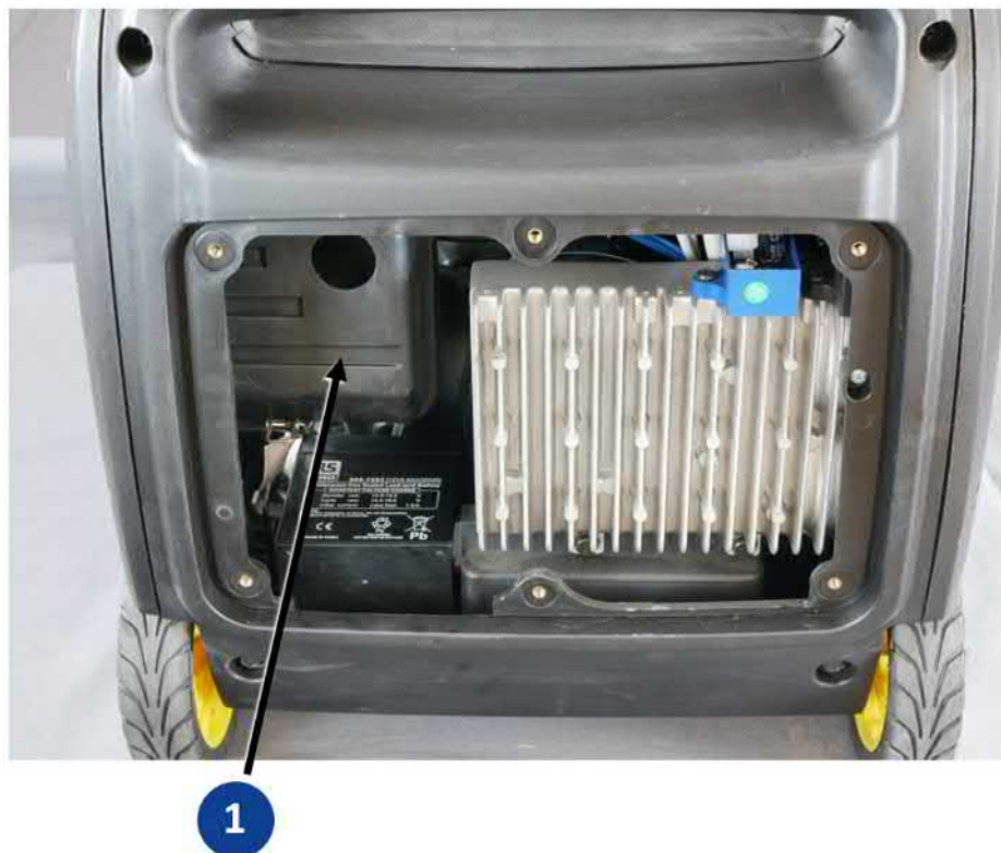
Fig. 9-5 Air filter behind the ventilation grille (removed)
