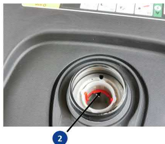
Fig. 7-2 Refuelling the generator
