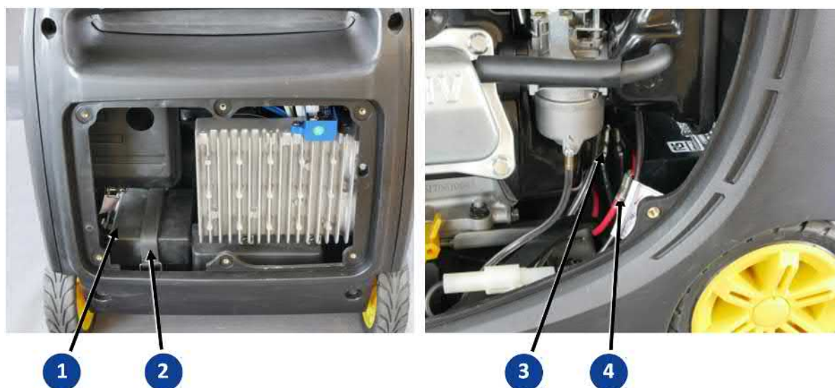
Fig. 9-9 Replacing the starter battery
