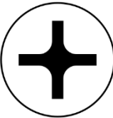
Screw: M2.5XL6 (D4.5) Screwdriver: Phillips PH00
