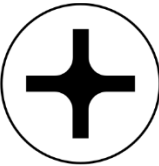
Screw: M2.5XL4 Screwdriver: Phillips PH00
