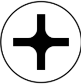
Screw: M2.5XL3 (D4.5) Screwdriver: Phillips PH00
