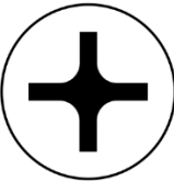
Screw: M2XL2.5 Screwdriver: Phillips PH00
