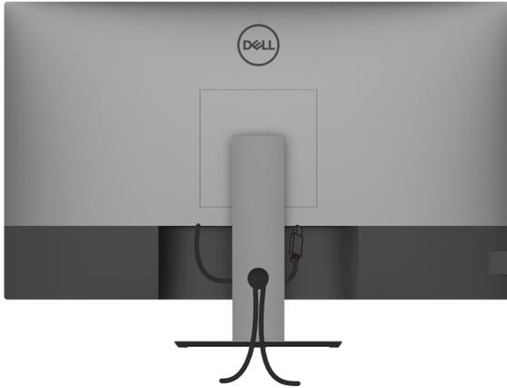
After attaching all necessary cables to your monitor and computer, (see [Connecting Your Monitor](#) for cable attachment) organize all cables as shown above.
