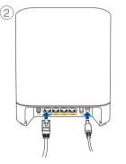
Connect the power cable and the network cable to the device.
