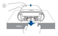
Pull downwards with two fingers to unlock the retention tab, and lift the device with the other hand.
