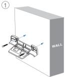
Drill two holes in the desired installation position on the wall and secure the wall mount stand.
