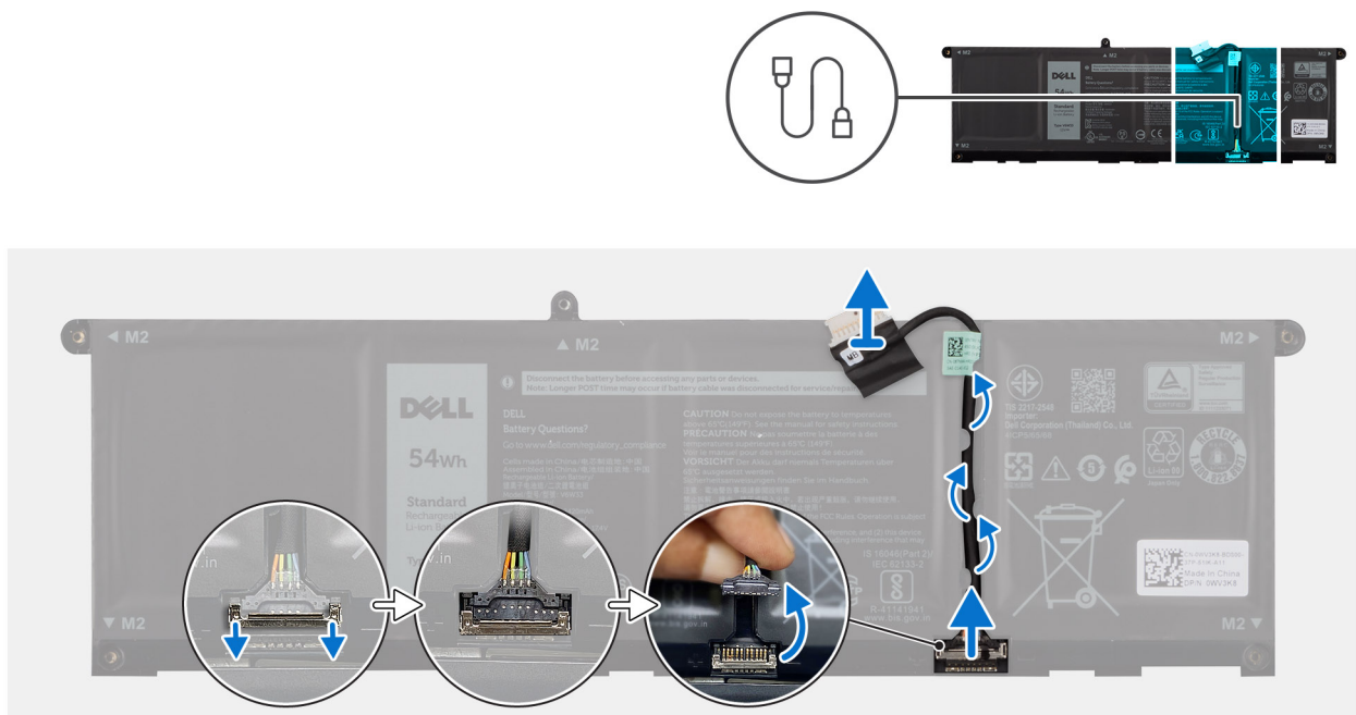
Figure 17. Removing the battery cable
