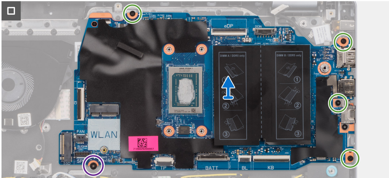
Figure 55. Removing the system board
