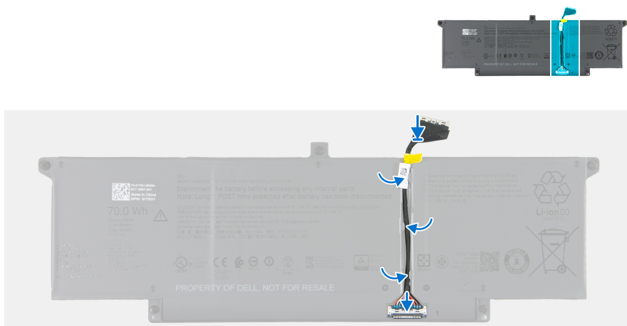
Figure 9. Installing the battery cable
