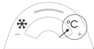
When the arm points to the right, you need to lower the temperature in the refrigerator compartment.
