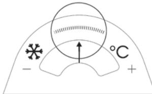
When the arm is in the middle, the temperature is ok.
