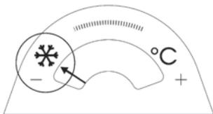
When the arm points to the left, you need to raise the temperature in the refrigerator compartment.
