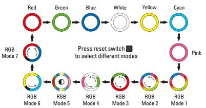
Press reset switch  $\blacksquare$  for 2 seconds to turn off the LED lights. When the LED lights are off, press reset switch  $\blacksquare$  to turn on the LED lights.
