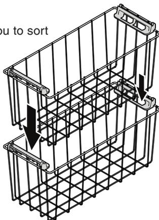
Press the handle downwards, lift and tilt inwards.
