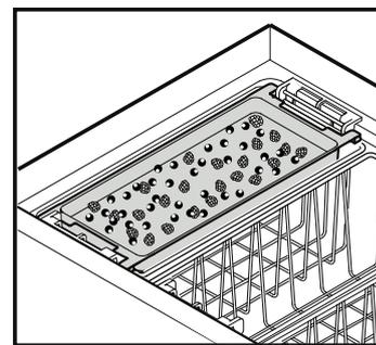
The freezer tray can either be suspended on the basket or can be slid into the interior container and used as a partition.
