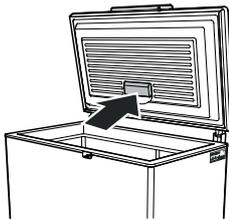
The light intensity of the LED light corresponds to laser class 1/1M.
