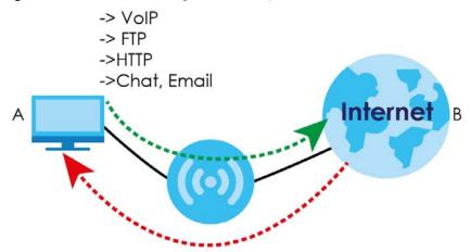
You can allocate specific amounts of bandwidth capacity (bandwidth budgets) to individual applications (like VoIP, Web, FTP, and Email for example).
