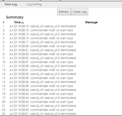
You can configure which logs to display in the View Log screen. Go to the **Log Setting** screen and select the types of logs you wish to display. You can enable the log server, to send detailed events to this server. Enter it's IP address or a Fully Qualified Domain Name (FQDN), and port. Then select the types of logs you wish to send to this server.
