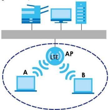
The wireless network is the part in the blue circle. In this wireless network, devices **A** and **B** are called wireless clients. The wireless clients use the access point (AP) to interact with other devices (such as the printer) or with the Internet. Your Zyxel Device is the AP.
