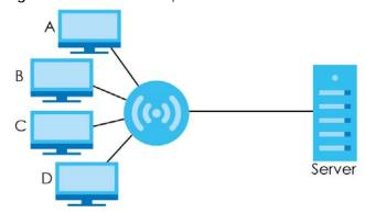
In the multicast example above, systems **A** and **D** comprise one multicast group. In multicasting, the server only needs to send one data stream and this is delivered to systems **A** and **D**.
