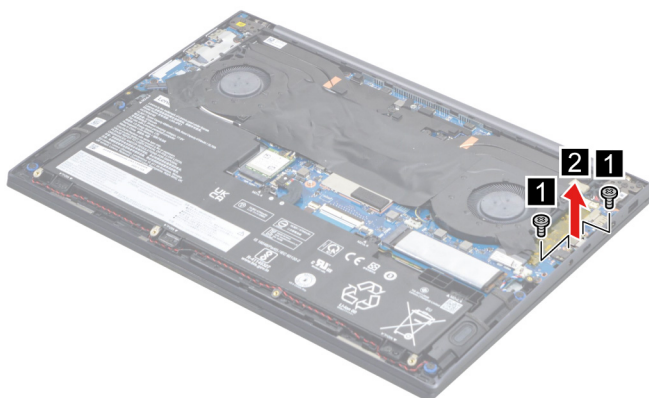
Figure 10. Remove the I/O bracket
