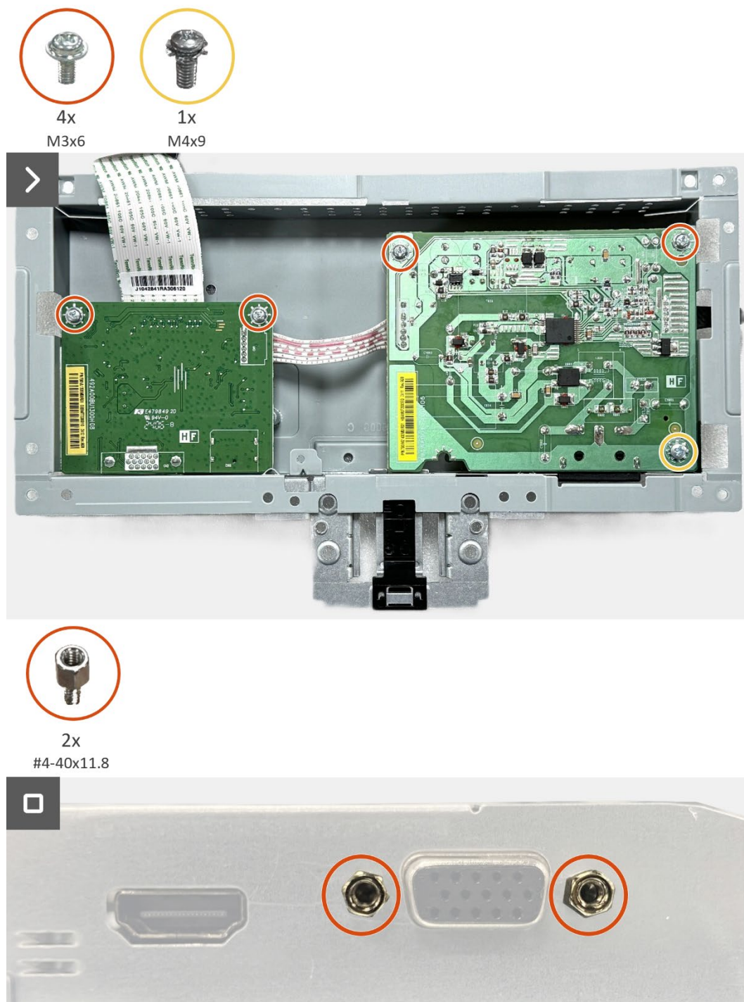
Figure 23. Installing the interface board
