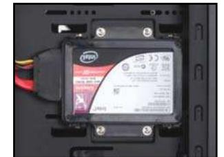
A 2.5" hard drive or SSD can be installed at a unique location.
