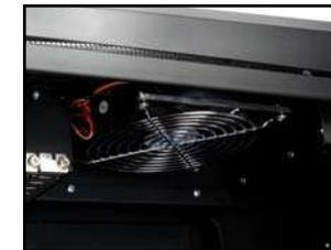
Top exhausting 120mm fan assist FT02's stack effect cooling.
