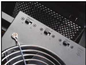
Three 180mm fans can be adjusted independently to run at 700rpm or 1000rpm.
